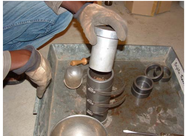
Figure 6: Special mold designed to prepare soil specimens according to AASHTO T 307 requirements
