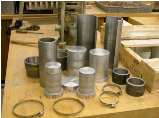
Figure 6: Special mold designed to prepare soil specimens according to AASHTO T 307 requirements
