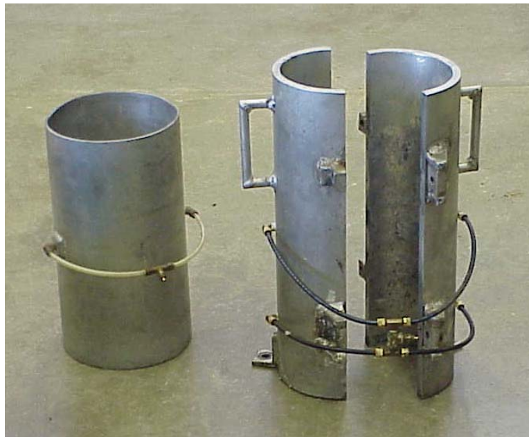
Figure 2. Split Mold Assemblies Used In Sample Preparation and Compaction
